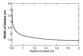
Figure 17. Variation of required width with radius for 1 kW power.
