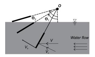
Figure 7. Side view of single blade of waterwheel during rotation.
