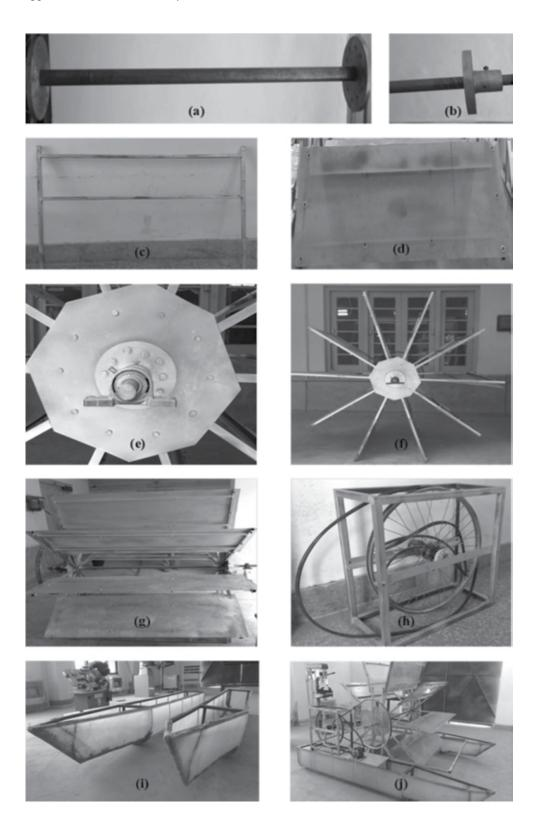
Figure 18. Fabrication of initial prototype floating waterwheel: (a) Shaft, (b) rotor collar, (c) blade frame, (d) blade made from fiber glass, (e) self-aligned roller bear on shaft, (f) fabricated rotor side view, (g) Fabricated rotor front view, (h) pulley box, (i) unfinished floats and (j) initial assembled prototype floating waterwheel.
