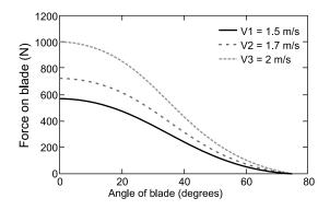
Figure 10. Force on blade during rotation of wheel's blade at different flow velocities.
