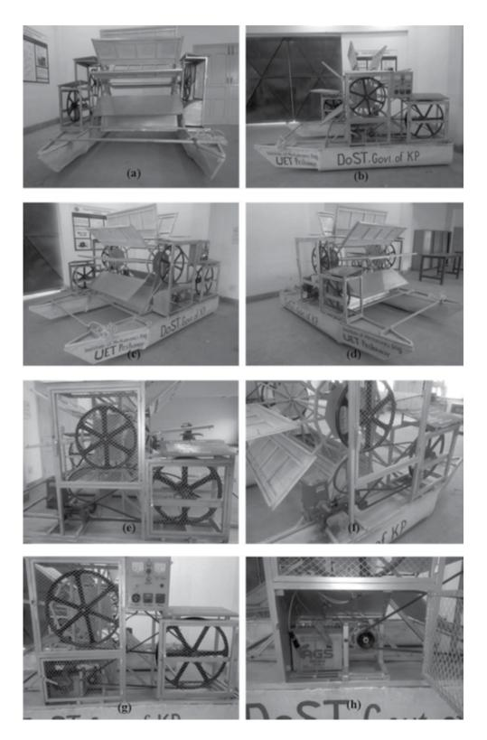
Figure 19. Fabrication of optimized prototype floating waterwheel: (a) Floating waterwheel front view, (b) side view, (c) right isomeric view, (d) left isomeric view, (e) pulleys and pump assembly, (f) pump close up, (g) pulleys and generator assembly and (h) battery and generator close up.
