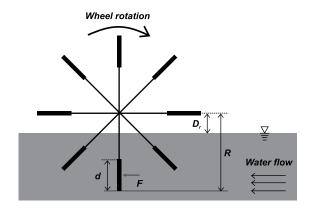
Figure 6. Side view of undershot waterwheel.
