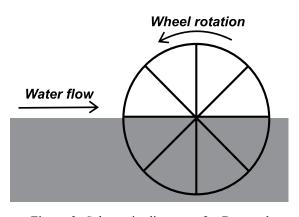
Figure 2. Schematic diagram of a Breast shot waterwheel
