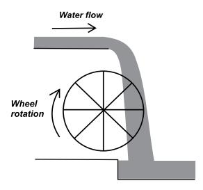
Figure 1. Schematic of overshot waterwheel.
