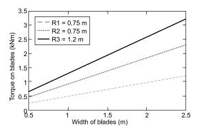
Figure 11. Torque as a function of blade's width at various radii of the waterwheel.
