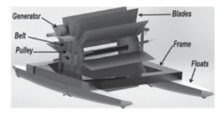
Figure 4. Solid model of floating undershot waterwheel.
