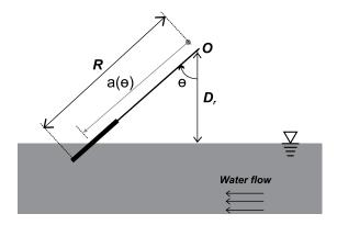
Figure 8. Rotation of the wheel as the blade starts leaving the water level
