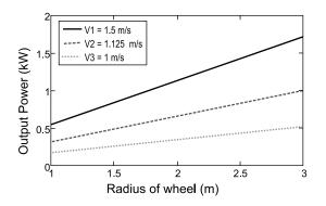
Figure 12. Variation of output power with flow velocity.
